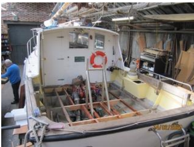
Stripped out and below new floor timbers ready to receive the new floor.
